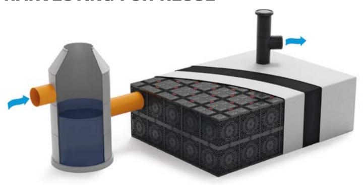
The rainwater running off from roofs or other surfaces and harvested for reuse is always channeled through a suitable pre-treatment stage before it can enter the storage tank.
