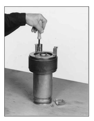
Using a socket wrench, fasten the feet (12) to the pump body (1) through the flange (5). (driving torque 5.5-6Nm)
