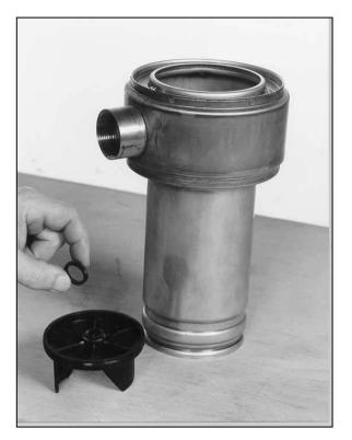
• Position the sandscreen V-ring (24) on the impeller (2); make sure that the squared side rests against the impeller.
