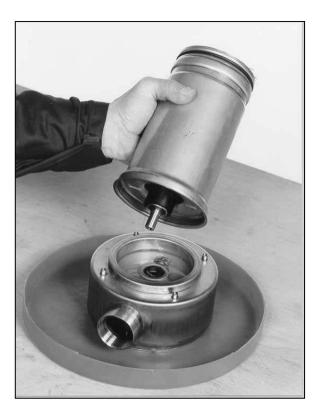
Remove the shell with stator after the oil residues have crained. Remove the fixed part of the mechanical seal (9) from the pump body.
