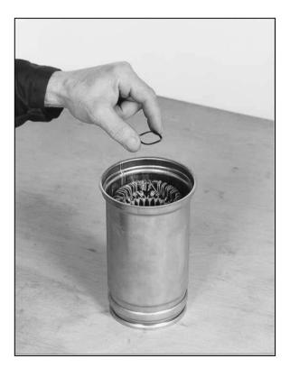
Remove the compensation ring (11) located in the bearing seat.
