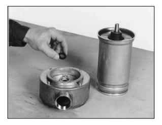
• Install the fixed part of the seal (9) in the pump body (1), with the polished side up. Be careful not to damage it.
