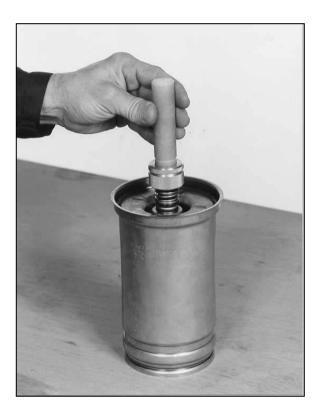
• With the plastic tap, position the rotating part of the seal in its seat as shown in the picture.
