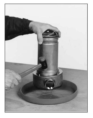
• Tap the pump body (1) gently with a rubber hammer to separate from the shell with wound stator (3).
