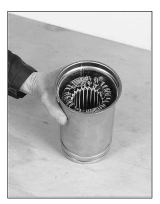
• View of motor casing with wound stator (3).
