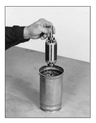
• Insert the rotor shaft with pre-assembled bearings (4).
