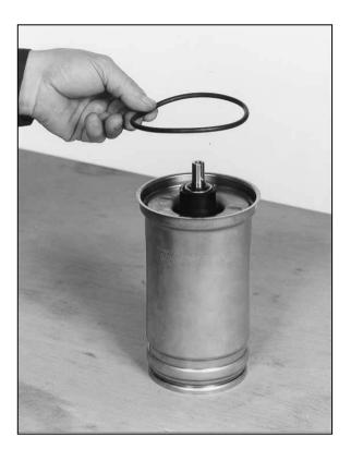
• Position the gasket (19) over the bearing's lower support.
