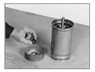
Insert the seal ring (21) over the bearing's lower support (6). During assembly make sure that the open side, where the spring is visible, is turned towards the inside of the bearing's lower support.
