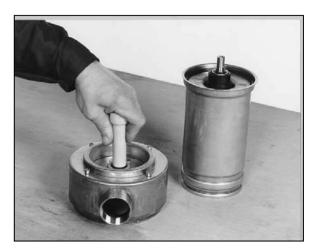
• With a plastic tap, slide the fixed part of the seal into position.
