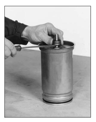
• Use a screwdriver to prize out the rotating part of the mechanical seal. Remove the washer underneath.
