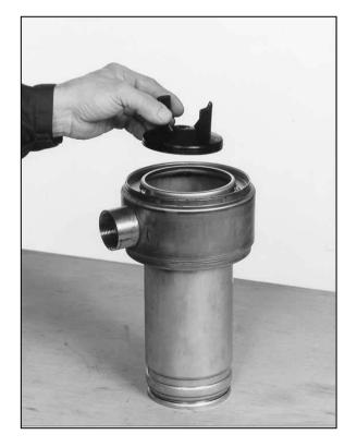
• For the DX 50 models: position the impeller lock tab in the shaft and install the impeller on the pump shaft.
