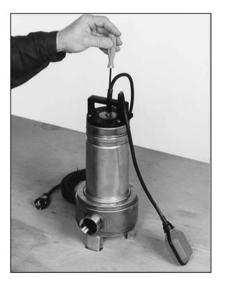
• Loosen the screw in the center of the head.
