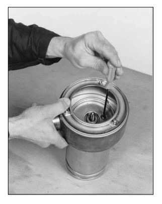
Fasten the screw with gasket (23). (driving torque 5-6Nm)
