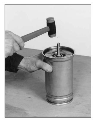
• Using a rubber hammer, gently tap the bearing's lower support on alternate sides to slide it into place.
