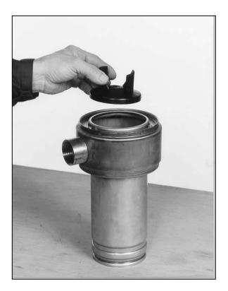
Remove the impeller (2); if necessary, use a pair of pliers. On the DX 10-15-20 models, retrieve the impeller lock tab. Remove the V-ring (24). Loosen the oil chamber fastening screw (23) and drain the oil.
