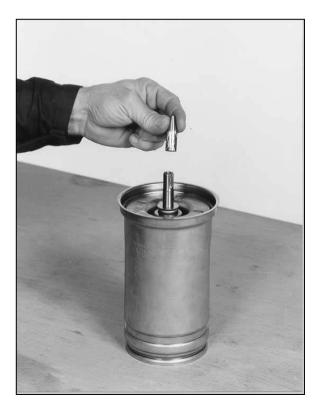
Put the mechanical seal's washer (9) on the pump shaft.
