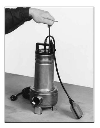
• Unscrew the three socket head screws from the head.
