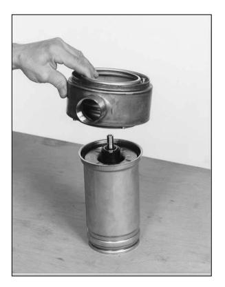
Carefully position the pump body (1) on the motor casing with wound stator (3).
