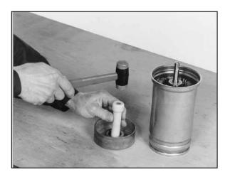
• With the plastic tap, position the lip seal ring in its seat in the lower support (6).
