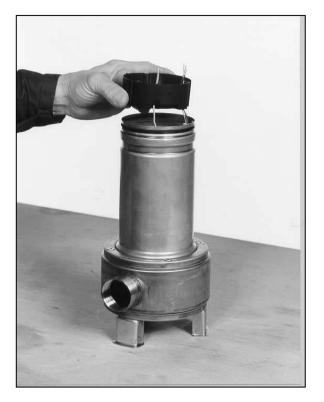
Install the electrical connection box (16), threading the wires through the holes.
