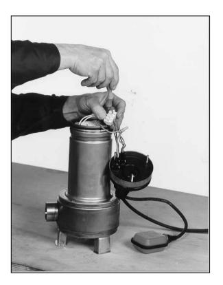
• Loosen the terminal box screws and disconnect all the wires, then remove the capacitor. (18 if any).
