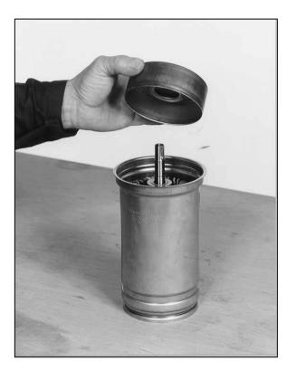
• Insert the bearing's lower support in the motor casing with wound stator.
