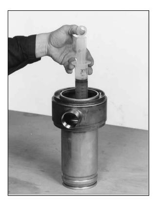
Place the pump upside down and add "Esso Marcol 82" oil slowly through the hole in the pump body, allowing the air to escape (quantity 0.080 liters).
