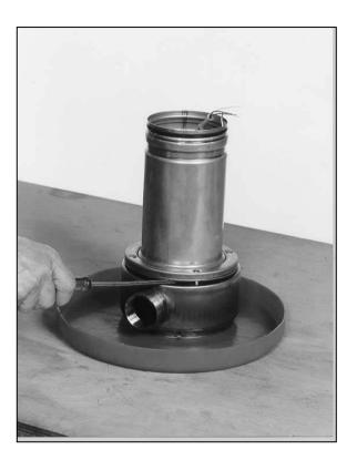
Remove the stop ring and place the pump in a pan to collect the oil. (if necessary, prize it out with a screwdriver).
