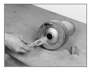
• With a socket wrench, loosen the screws that hold the feet (12).
