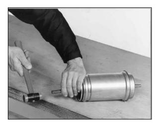
• Tap the shaft gently (4) on the head side, through the hole in the bearing seat.
