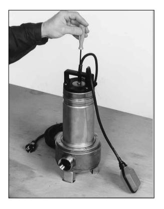
Fasten the screw in the center of the head and make sure that the O-ring is in place. (driving torque 5-6Nm)
