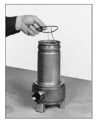
• Turn the pump upside down and install the gasket (19) in its seat in the motor casing with wound stator.
